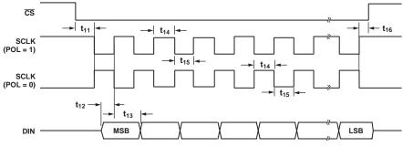
Figure 19. Write Cycle Timing Diagram
