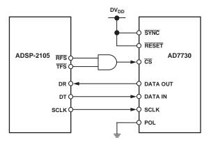
Figure 22. AD7730 to ADSP-2105 Interface
