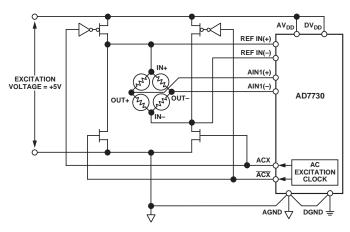
Figure 8. Ratiometric Generation of Reference in AC-Excited Bridge Application
