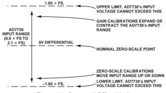
Figure 16. Span and Offset Limits
