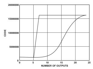
Figure 15. Step Response for FASTStep and Normal Operation
