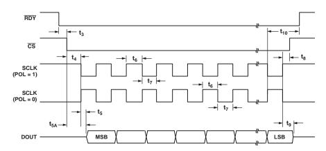
Figure 18. Read Cycle Timing Diagram
