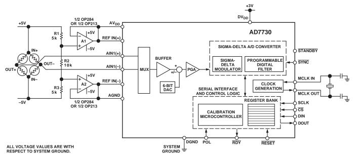
Figure 25. AD7730 with Bipolar Excitation of the Bridge
