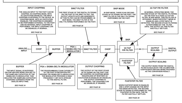
Figure 3. Signal Processing Chain
