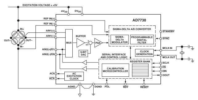
Figure 23. Typical Connections for DC-Excited Bridge Application
