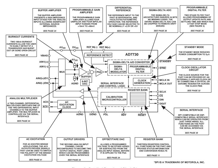
Figure 2. Detailed Functional Block Diagram
