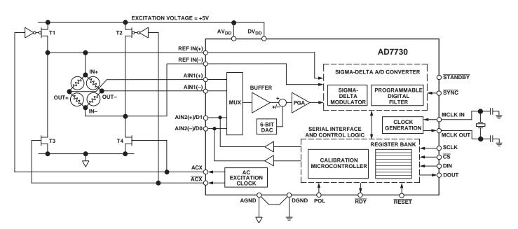
Figure 24. Typical Connections for AC-Excited Bridge Application
