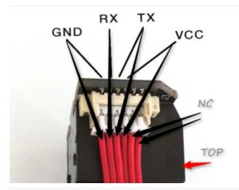
If your sensor has all the same-color wires, The first wire from the left is ground, then the two data pins, then power. You'll have to cut, strip and solder the wires.
