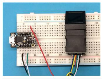
Every CircuitPython board has a hardware UART. Check the product page or look for **RX** and **TX** written on the board. Remember that the RX from the sensor goes to the TX on the board! If you have problems try swapping them, its a common mistake
