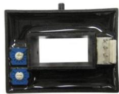
Open loop current sensor based on the principle of Hall-effect. It can be used for measuring AC,DC,pulsed and mixed current.
