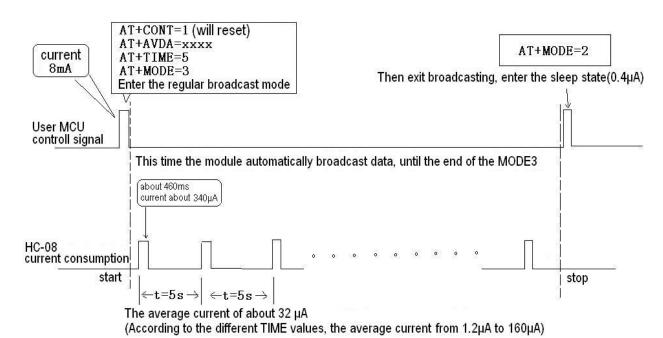
The user MCU to the module of UART port to send 10 bytes hexadecimal code of "0xFF, 0xFF, 0xFF" to awaken the module, module into the full power mode. At this point the user can reasonably set according to need, the above "AT+CONT=1, AT+AVDA=xxxx, AT+MODE=3, AT+TIME=5" set to: broadcast and can not connected, the broadcast data is XXXX, mode3(period of 5).
