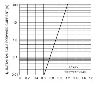
V<sub>F</sub>, INSTANTANEOUS FORWARD VOLTAGE (V) Fig. 2 Typical Forward Characteristics (per element)
