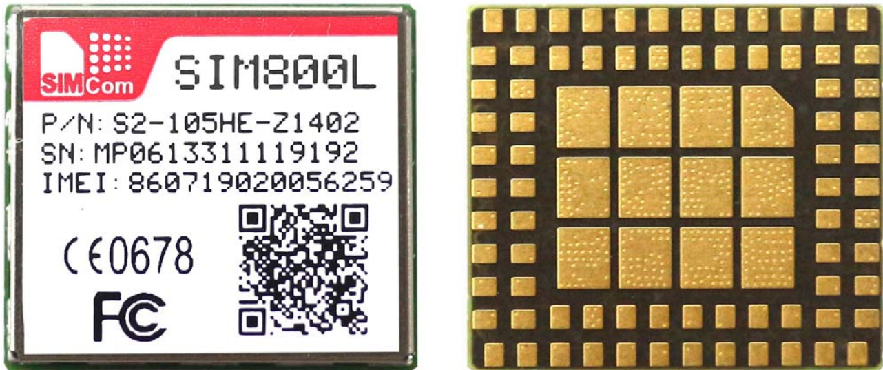
Figure 53: Top and bottom view of SIM800L
